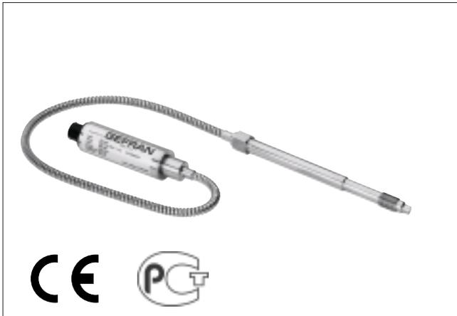
The M3 series of Gefran, are pressure transducers for using in High temperature environment. The main characteristic of this series is the capability to read temperature of the media up to 400°C. The constructive principle is based on the hydraulic transmission of the pressure. The fluid-filled system assures the temperature stability. The physical measure is transformed in a electrical measure by means the strain-gauge technology.
